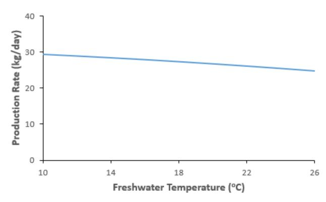
Lower temperatures on the freshwater side enhance the production rate
