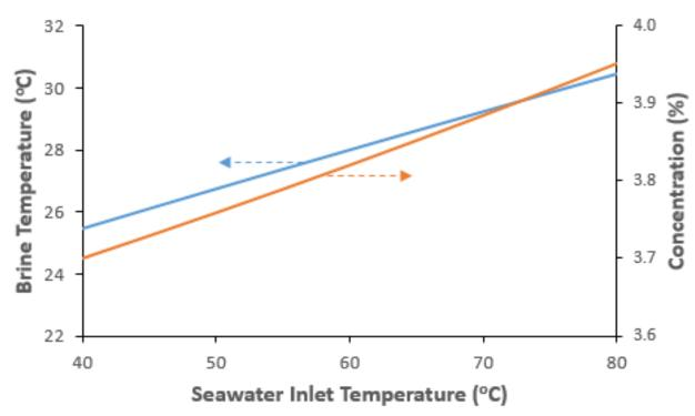
Higher temperatures results in elevated brine temperature and concentration which are both environmental hazards
