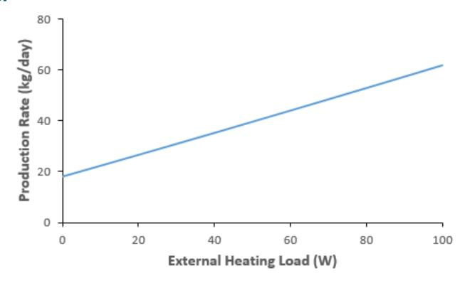
Using 100 W of external heating load (other than the feed heating) provides up to 4 times better production rates
