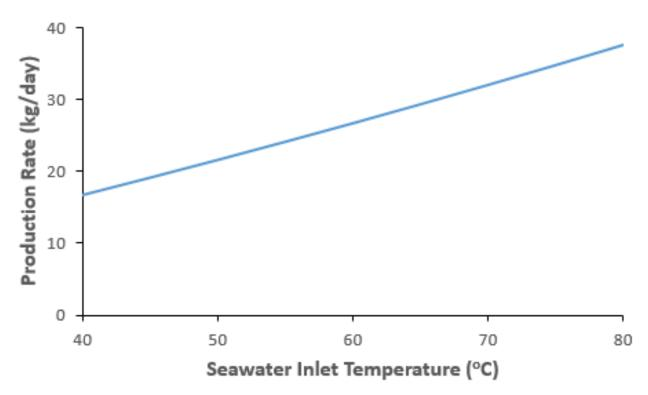
Production rates of around 40 kg/day are calculated for inlet temperature of 80 °C
