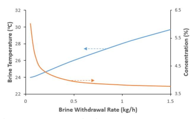
Low brine rates cause higher concentrations increasing scaling hazards
