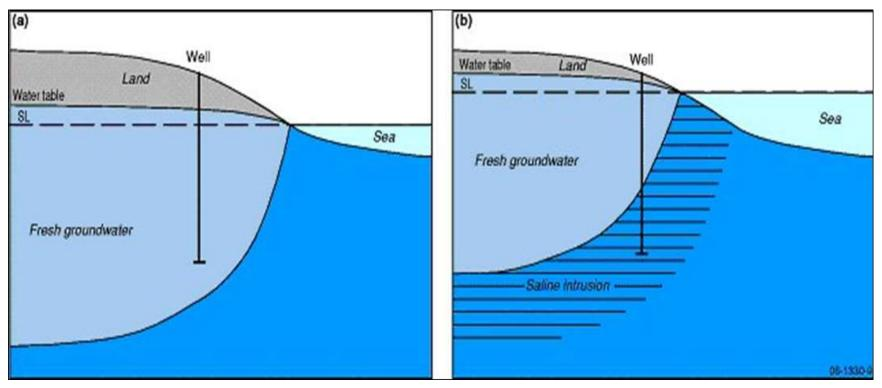
The effect of sea level rise on freshwater aquifers. (a) The baseline situation, where the bottom of a well is in fresh groundwater. (b) The impact of sea level rise, resulting in the bottom of the well being in saline water.
