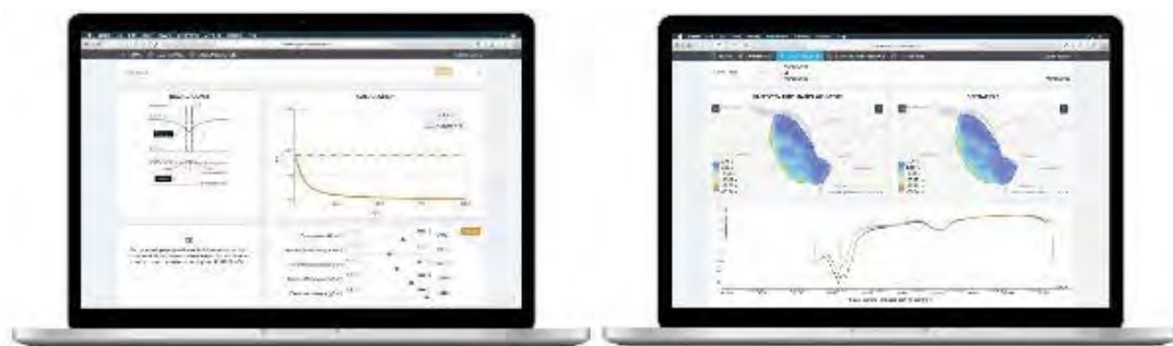
Fig. 5. Screenshots of simulation tools included in the INOWAS platform. Left: analytical tool for the calculation of saltwater upconing under a pumping well (Glass et al., 2018a). Right: scenarios analysis of a MODFLOW-based groundwater model (Glass et al., 2018b).
