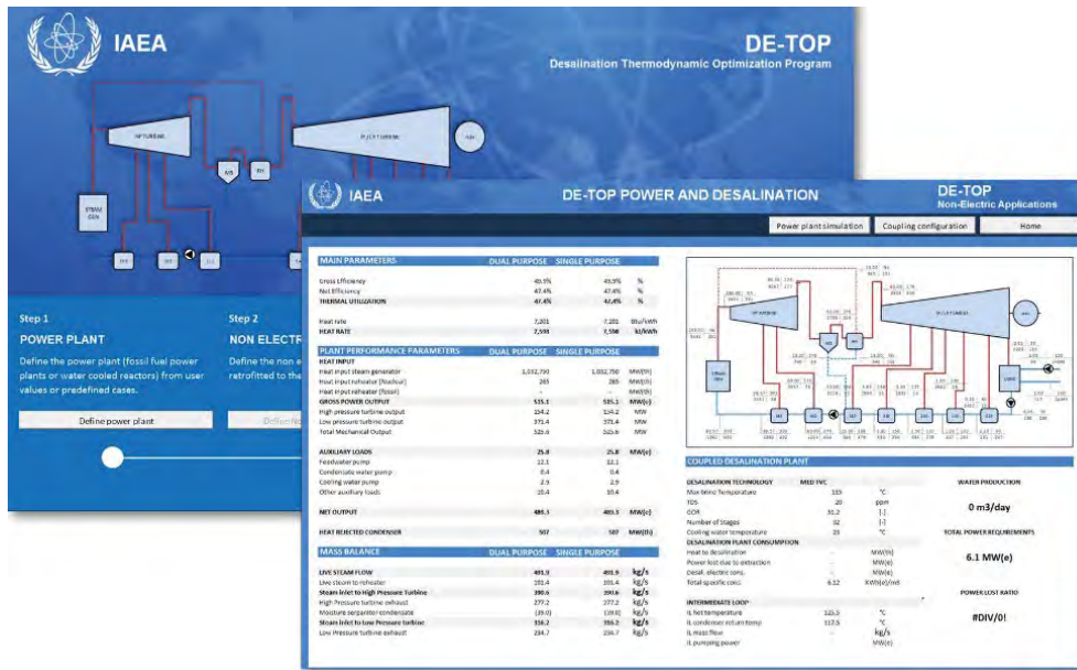
Fig. 2. Interface of the IAEA desalination thermodynamic optimization program (DE-TOP).
