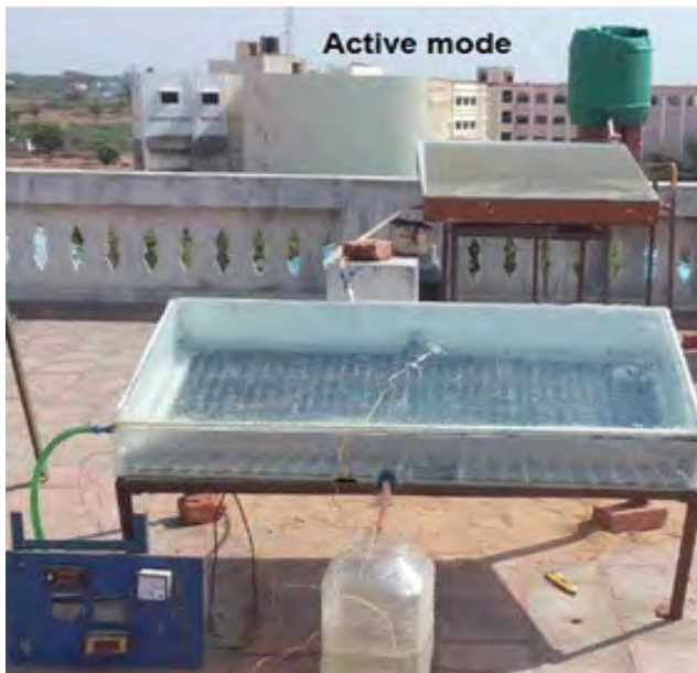
Fig. 2. Photographic view of the ISPB still integrated with the STC.
