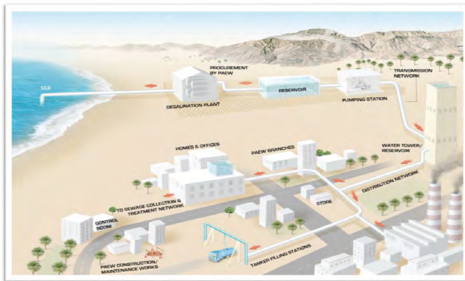
Fig. 1. Water supply system in Oman.
