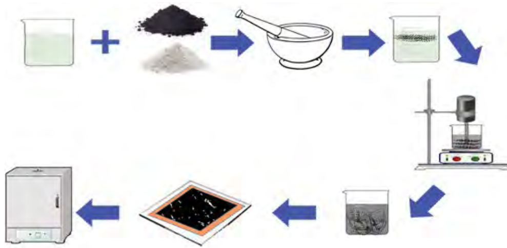
Fig. 2. CNT membrane fabrication.
