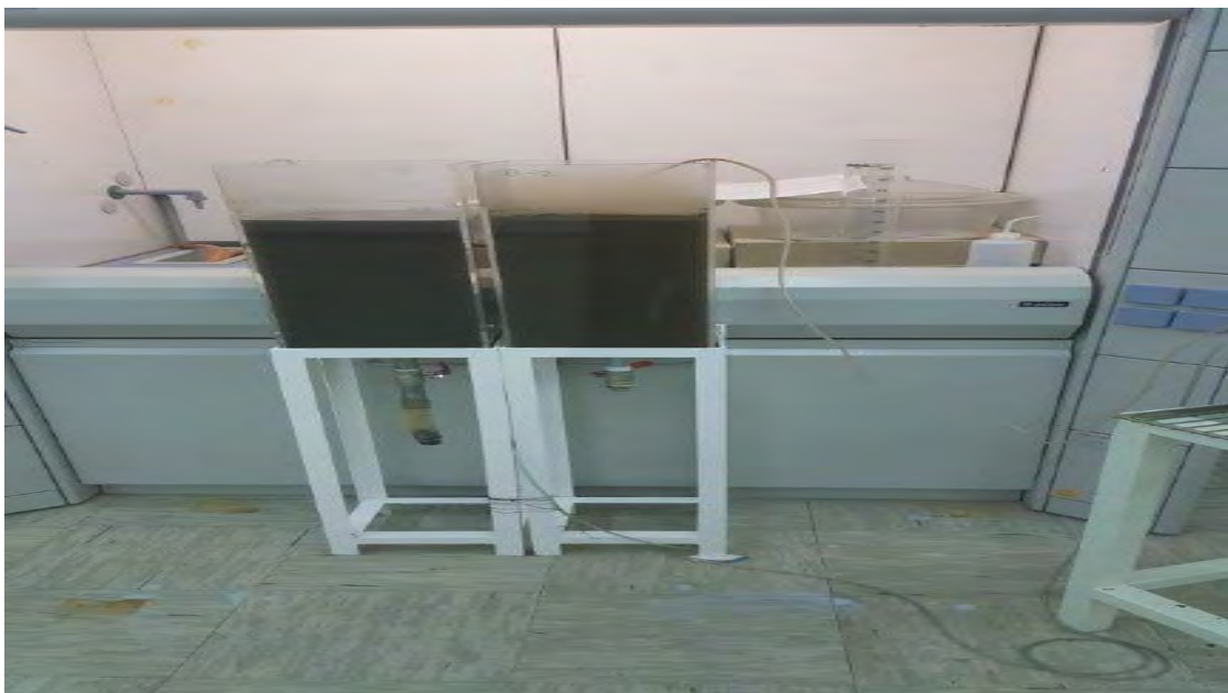
Plate 1. Bioreactors for aerobic treatment of wastewater.
