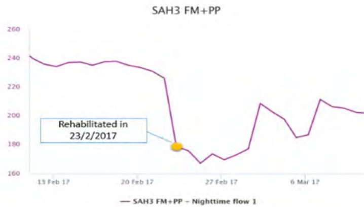
Fig. 15. Reduction in water losses by pipes rehabilitation.
