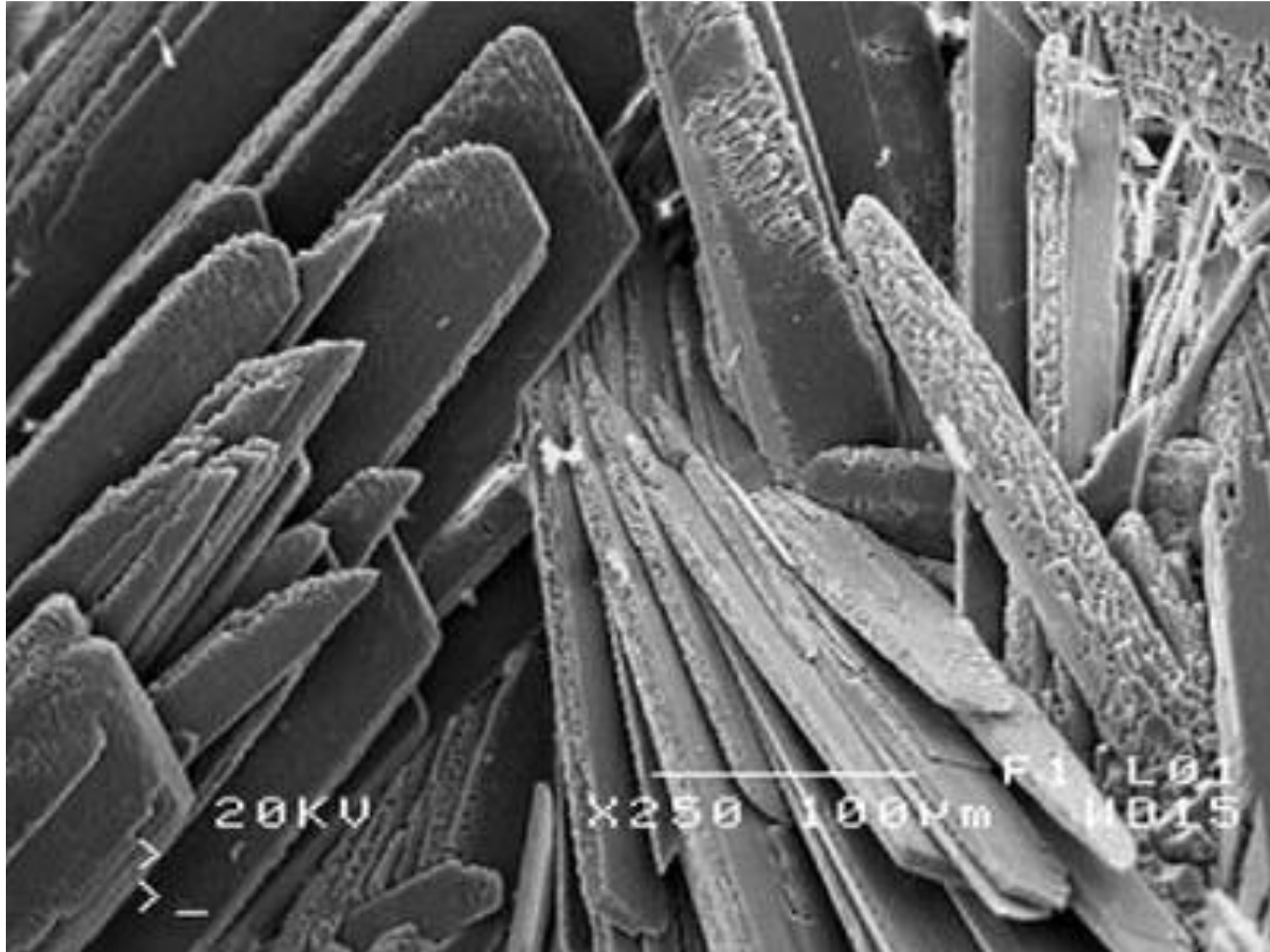
SEM image of calcium sulfate deposit on the membrane surface during the MD process.
