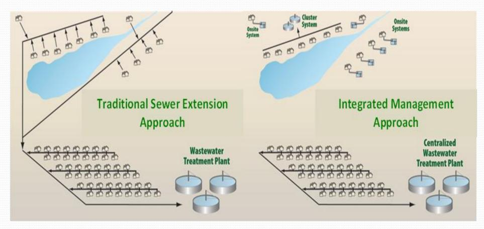
Traditional sewer extension and integrated management approach that uses a variety of system scales to provide treatment that matches the context, based on D'Amato, Striano, Moeller (2011).
