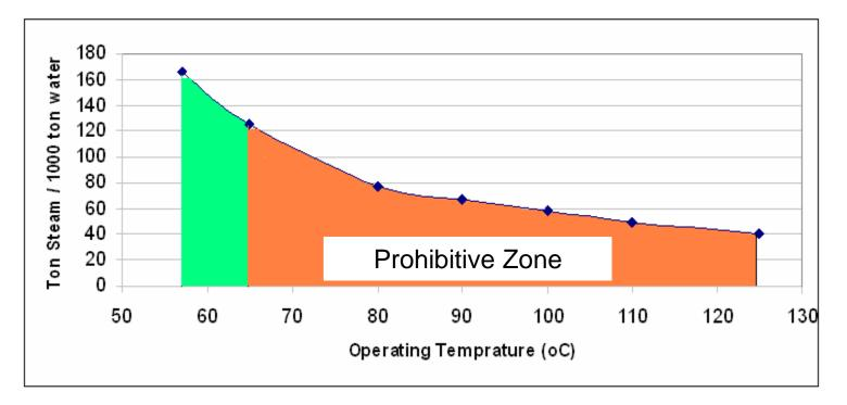
Impact of the variation of operating temperature on the energy consumption of the MED Process
