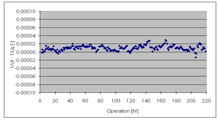
The fouling factor of the high temperature (cell# I) when operated at a maximum temperature of 125°C, was virtually constant and there was no sign of deterioration.
