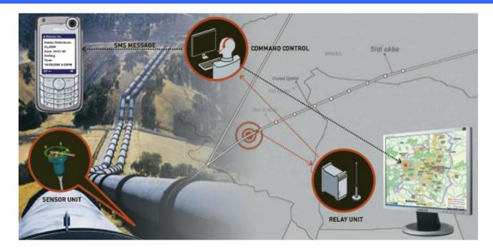
The sensors connect to the central control room which is able to detect, classify and monitor :
