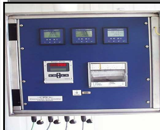
Automatic water quality monitoring station`
