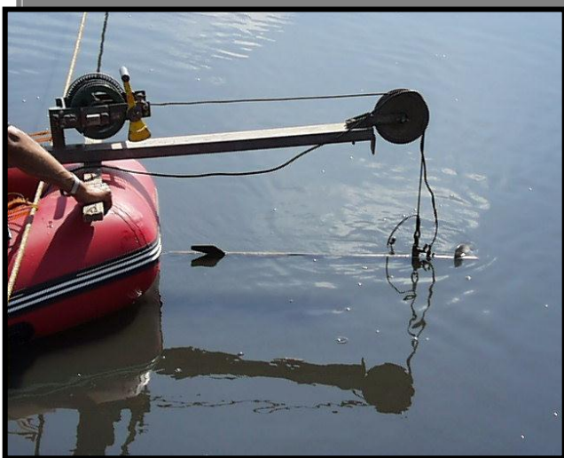
Discharge measurement using current meter
