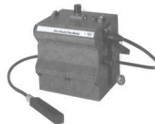
Figure 2-9: Isco 2150 Area Velocity Flow Logger
