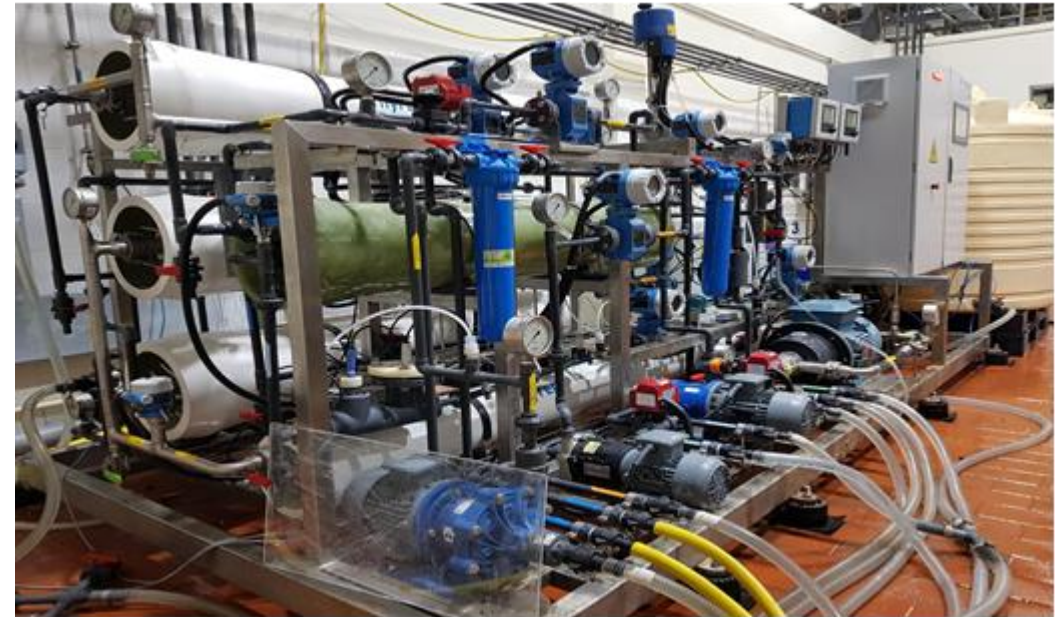
Image of the FO-RO Pilot Test Unit at KISR
