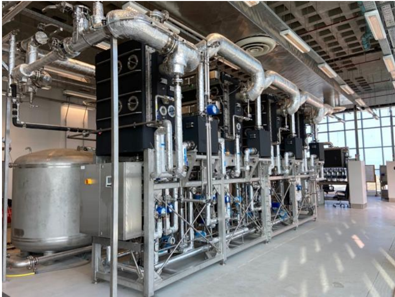
Image of the MED Pilot Test Unit at KISR
