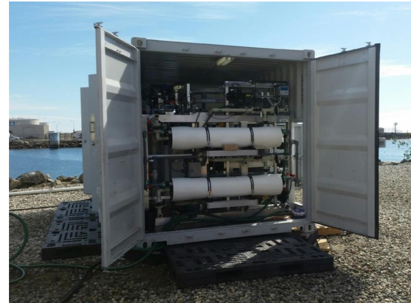
Image of Commercial-Scale FO Membrane Modules
