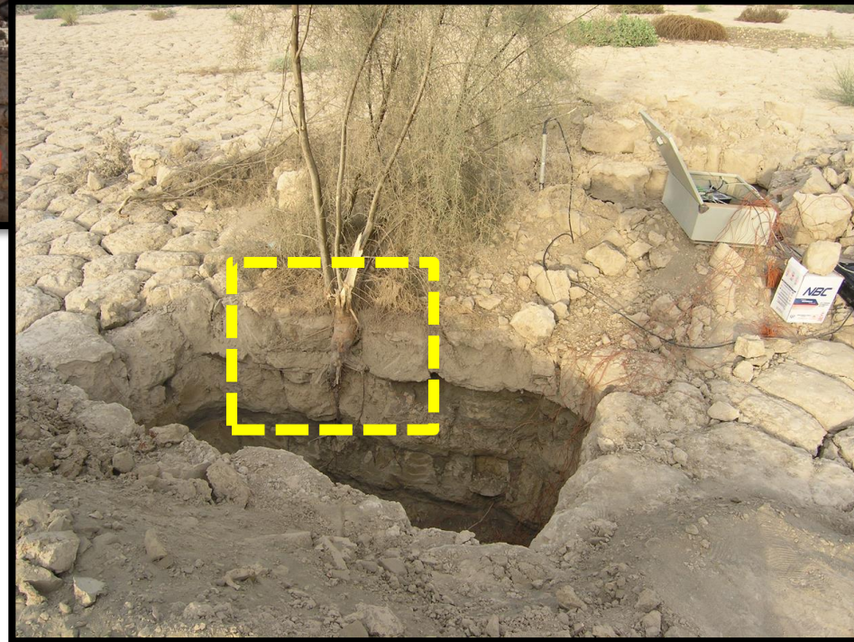
Al-Maktoumi, A., Kacimov, A., Al-Busaidi, H., Al-Ismaily, S., Al-Mayahi, A., Al-Khanbashi, S., and Al-Sulaimi, A. Enhancement of infiltration rate of clogged porous beds in the vicinity of dams in arid zones by the roots of indigenous Ziziphus spina-christ trees. Hydrological Processes , 2020, v. 34, 4226–4238
