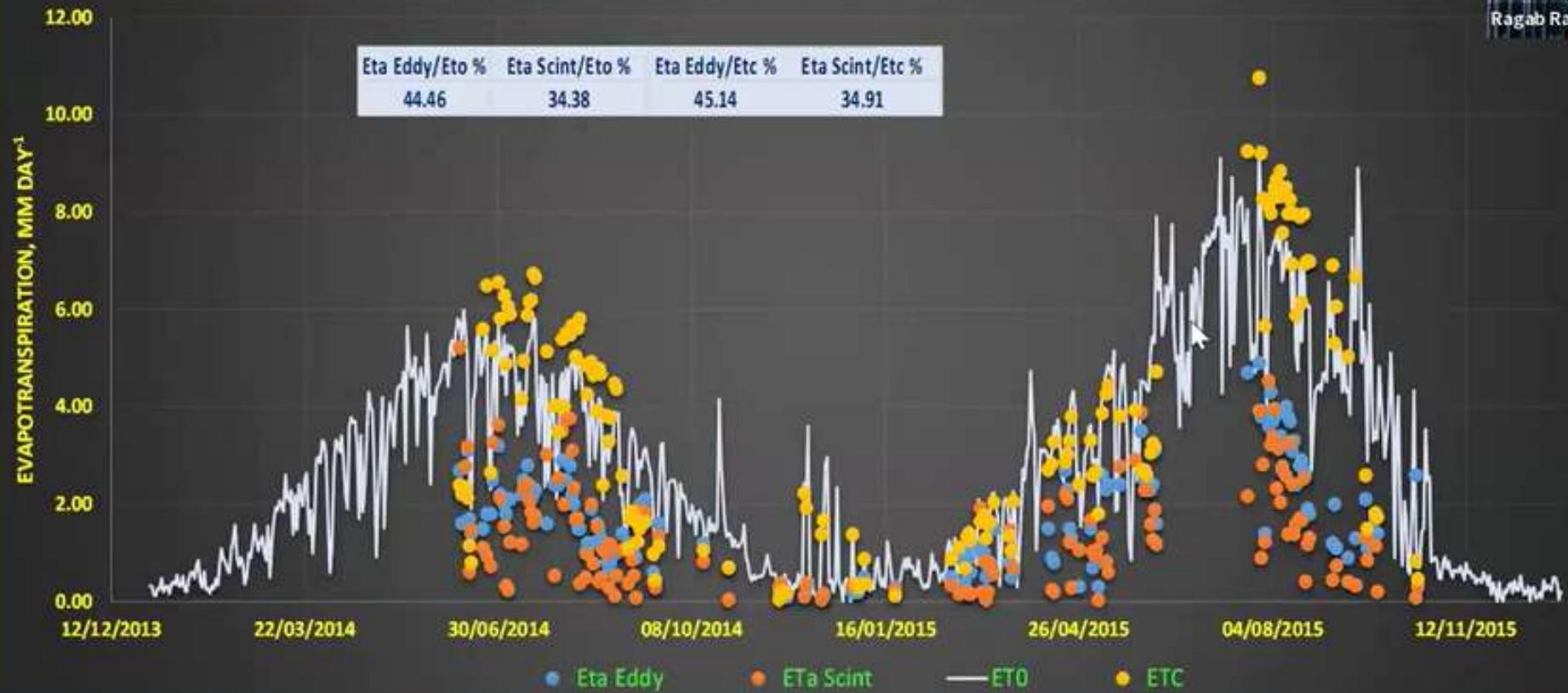
**Comparison between actual evapotranspiration measured by Eddy Covariance and Scintillometer, reference evapotranspiration estimated from Penman-Monteith equation and crop evapotranspiration calculated from ETo and the weighted mean of the crop coefficient Kc.**
