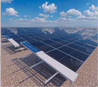
Solar PV Cleaning Robot
