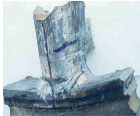
Figure 17. Photograph of cut up portions of intermediate bearing support block shows the cracks at arms and rim interface.
