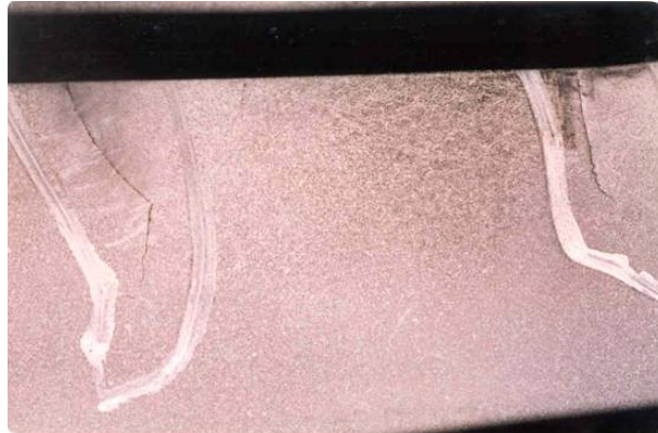
Figure 21. Photograph of blade No. 4, stage 9, three cracks are visible
