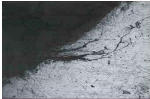
Figure 5. Photomicrograph taken from near the edge of specimen showing the emanation of fine, branching cracks from the corroded edge
