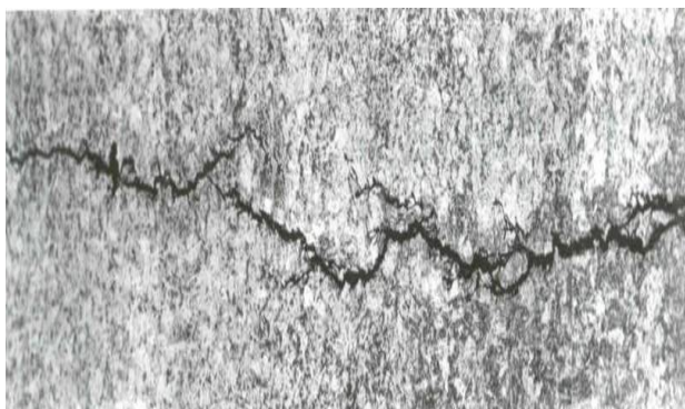
Figure 24. Photomicrograph of crack # 3 of blade# 4 multiple branched cracks are visible, which are both transgranular & transgranular 280X
