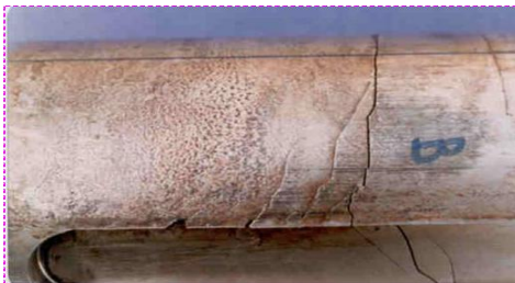
Figure 1. Cracks on the shaft of a brine recirculation pump
