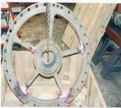
Figure 16. Photograph of main seawater pump intermediate bearing support. Arrows indicate the area where cracks have developed during service
