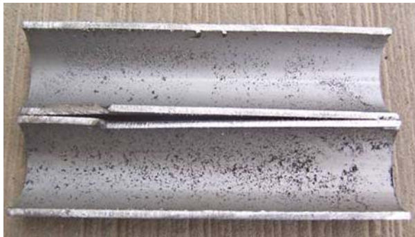
Figure 13. Splitted tube showing oil deposits inside
