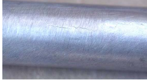
Figure 12. Crack propagation horizontally along the tube
