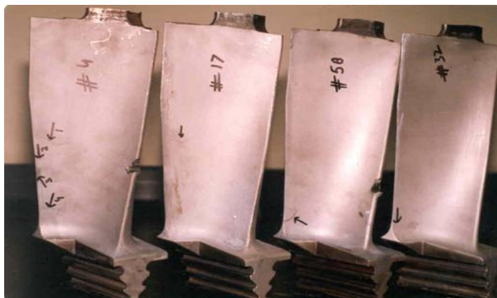
Figure 22. Four cracked blades from 9 th Stage of turbine #81
