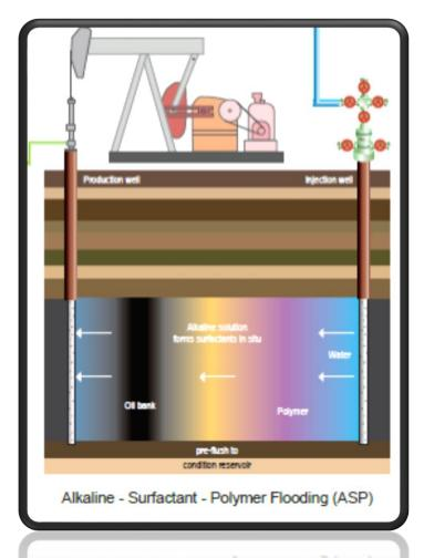
Alkaline - Surfactant - Polymer Flooding (ASP)
