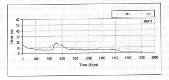
Figure 7: Observed and simulated hydrographs of wells BHF-1 and BHF-9, calibration period.
