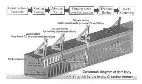
Figure 4: Construction procedure of continuous cut-off
