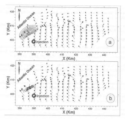
Fig. 5: Hydrodispertive modelling in the Mamora groundwater near the coastal line (a. Upwind method, b. Superbee method).
