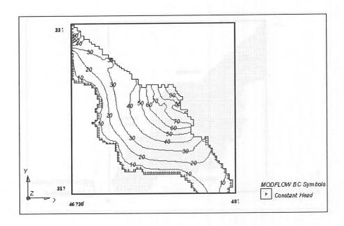
Fig. (12): Water Level Contour Map after One Year Simulation.
