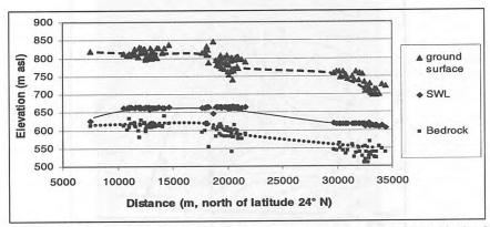
Figure 5: S-N cross section of ground surface elevation, static water level, and bedrock elevation across the study area as obtained from well completion reports.
