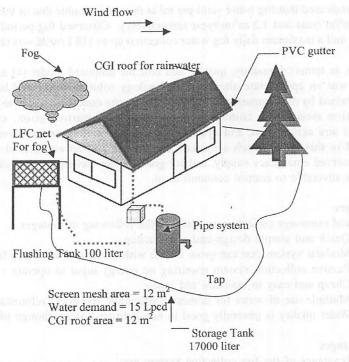
Figure 4: Rural Model House with Fog and Rainwater Collection System
