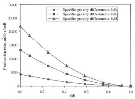
Figure 8 Relationship between d/h and critical production rae from a horizontal well in the studied Saudi groundwater aquifer at various specific gravity difference.
