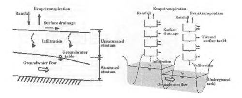
Figure 6: Image of storage tank model
