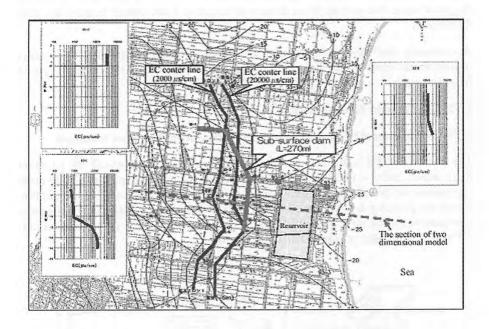
Figure 15: The observed electric conductivity contour line and the section of twodimensional FEM analysis model
