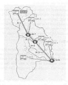
Fig. 5: Schematic basin model of Wadi Ham.
