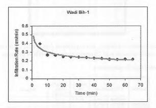
Figure 5: Infiltration rate curve at site one, Wadi Al Bih. 7
