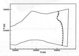
Figure 6. Position of the interface toe (scenario 2). Present model (dashed and solid lines for sets 1 and 2 respectively) and Larabi and De Smedt (1997) model (dash-dot line).
