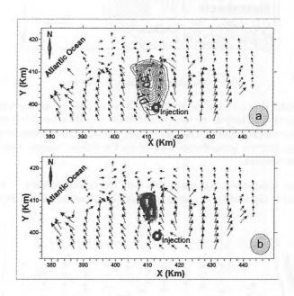
Fig. 4: Hydrodispertive modelling in the Mamora groundwater far from the coastal line (a. Upwind method, b. Superbee method).
