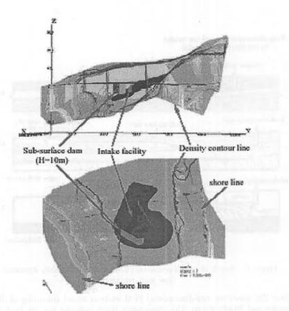
Figure-18 Result of three-dimensional FEM analysis by density-dependent flow mass transport
