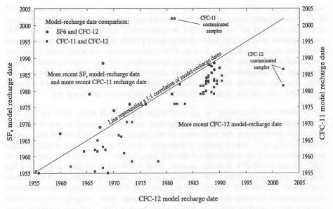
Figure 4. Comparison of CFC-12 and SF<sub>4</sub> estimated model-recharge dates for 17 ground-water samples from the surficial aquifer and CFC-12 and CFC-11 estimated model-recharge dates for 54 ground-water samples from the surficial aquifer.
