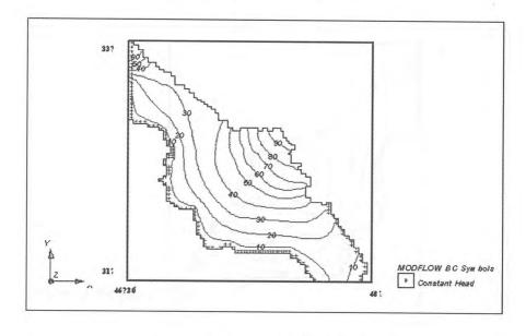
Fig. (11): Steady-State Simulation of the Aquifer.
