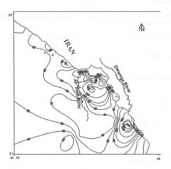
Fig. (7): Aquifer Transmissivity map (m²/d).
