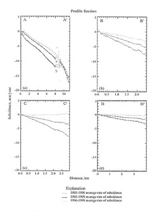
Figure 5: Rate of land-surface deformation determined by InSAR for the profiles found in Figures 2, 3 and 4 are shown.
