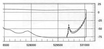
Figure 7: Vertical cross-section through pumping well W1 showing the interface position (scenario 2). Present model (dashed and solid lines for sets 1 and 2 respectively) and Larabi and De Smedt (1997) model (dash-dot line).
