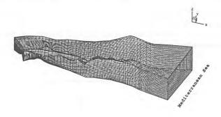
Figure 4: 3-D structured mesh of Oued-Laou aquifer
