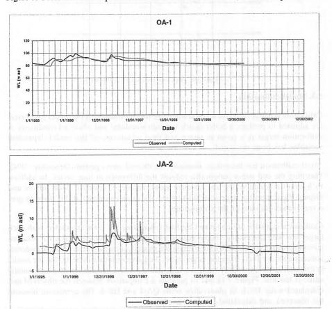
Figure 8: Observed and computed water levels for wells OA-1 and JA-2, validation period.
