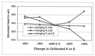
Figure 7: Sensitivity analyses where changes in simulated 1992 head are plotted versus changes in calibrated K and S.
