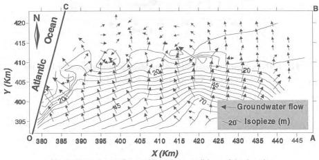
Fig. 3: Groundwater flow and boundary conditions of the domain.
