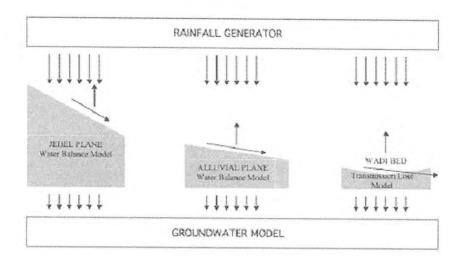
Figure 3 Schematic of distributed wadi water resource model
