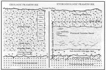
Figure 2: Correlation between geologic and hydrogeologic frameworks in northern Harrat Rahat
