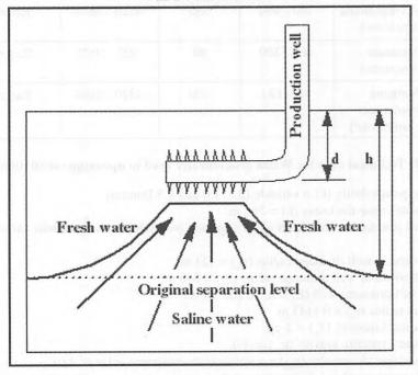
Figure 2 A schematic diagram of upconing phenomenon in a horizontal well.
