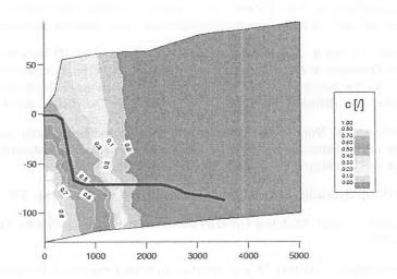
Figure 12: Measured salt freshwater interface (black line, from geophysical investigations) and computed isosaline c [/] contours.
