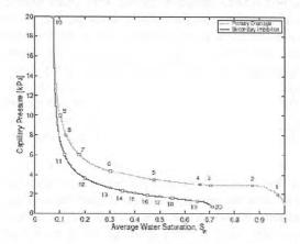
Figure 3: Gas injection after *o/w* primary drainage or secondary imbibition with different initial saturations (denoted by the squares)
