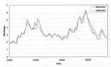
Figure 5: Hydrographs of measured and calibrated base flow discharges in m<sup>3</sup>/s
