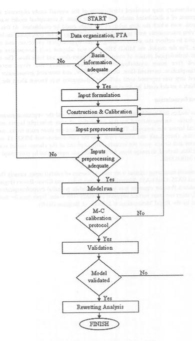
Figure 2: Multi-step modeling procedure
