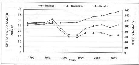
Figure 7: Leakage Rate in the Transmission and Distribution Networks [10]
