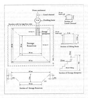
Figure 2: Layout Plan of Rainwater Harvesting System
