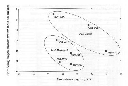
Figure 5. Relation of ground-water age and sampling depth for 7 ground-water samples from from wells in the Al Jaww Plain.
