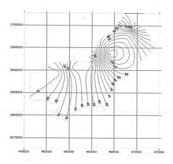
Figure 6: Aquifer thickness contour
