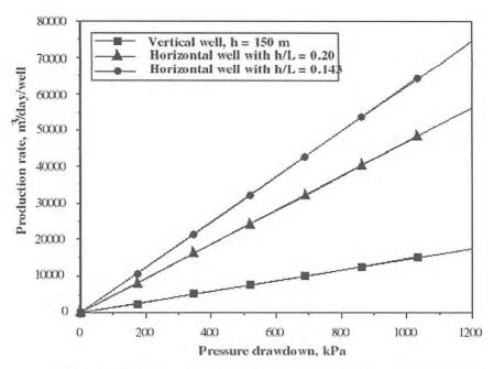
Figure 7 Relationship between pressure drawdown and productio rates from vertical and horizontal wells.
