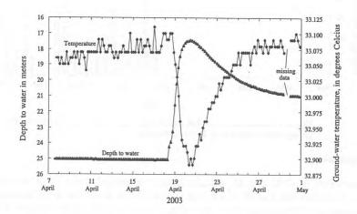
Figure 6. Depth to water and ground-water temperature in well GWP-258 in the Al Jaww Plain, 7 April 2003 to 1May 2003.
