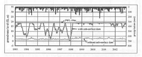
Figure 11: Simulation results of BLOCK 6-2 with and without a sub-surface dam
