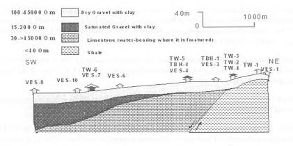
Figure 6: Geoelectric subsurface cross section along the SW-NE direction
