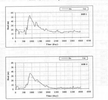
Figure 8: Observed and simulated hydrographs of wells BHF-1 and BHF-9, validation period.
