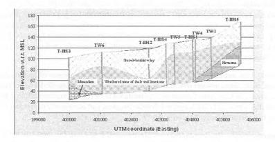
Figure 3: Lithological cross-section along selected boreholes (Modified from ENTEC, 1998). For borehole locations see Fig.1.
