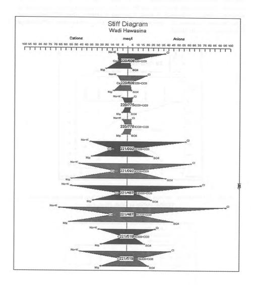
4: Stiff diagram showing groundwater chemistry for 1994 and 2002. Polygons for the same well are staked so that 1994 is on top of 2002 polygon.
