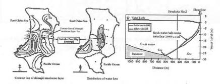
Figure 12: Foundation contour line and fresh water lens in the Tukenjima-iland
