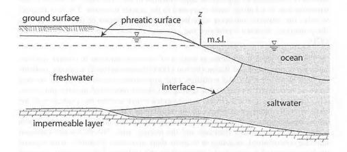
Figure 1: Schematic sketch of saltwater intrusion, sharp interface model.
