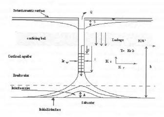
Figure 3. Saltwater upconing beneath a well
