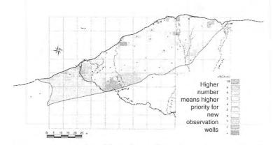
Fig. 3: The most important places to start constructing a new set of peizometers .
