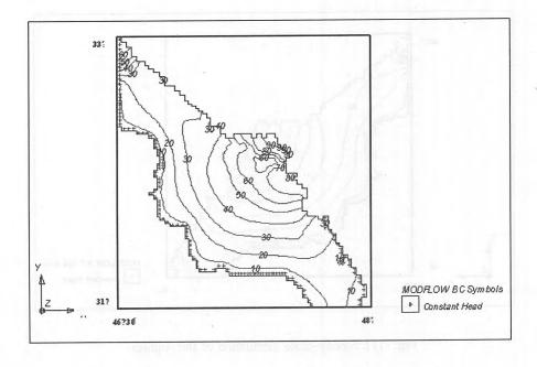
Fig. (13): Water Level Contour Map after Five Years Simulation.
