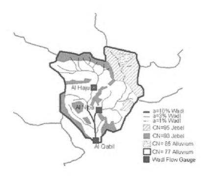
Figure 4 Distributed parameters for wadi water resource model, Wadi Ghulaji, Sultanate of Oman
