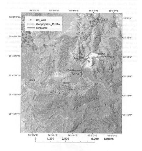
Figure 1: A recent satellite image of the studied area in Wadi Al Bih with the locations of monitoring wells, a production well and geophysical profiles.
