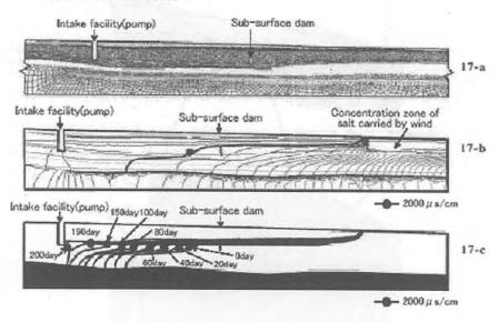
Figure 17: Result of two-dimensional FEM analysis by density-dependent flow mass transport
