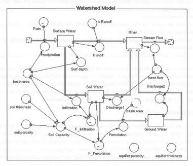
Figure 3: Typical hydrologic model of a watershed (<a href="http://www.acad.carleton.edu/curricular/GEOL/DaveSTELLA/Water/watershed/2.gif">http://www.acad.carleton.edu/curricular/GEOL/DaveSTELLA/Water/watershed/2.gif</a>) from "Modeling Water flow in a Watershed"
