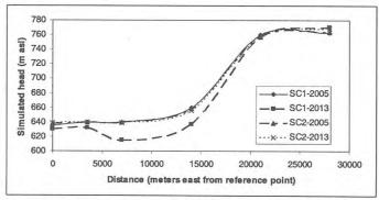
Figure 9: Water table across the wellfield (W-E) as simulated in scenarios 1 and 2, for 2005, and 2013.
