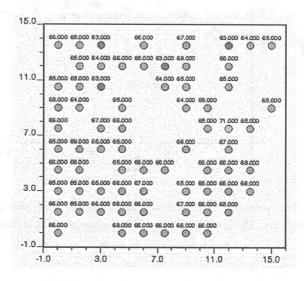
Figure 2: Plan view of the "imaginary monitoring wells - IMW". The number on top of each IMW indicates the DGW surface detected by the GPR.
