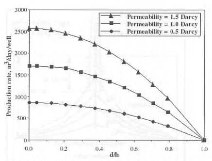
Figure 5 Relationship between d/h and critical production rate from a vertical well in the studied Saudi groundwater aquifer at various permeabilities.
