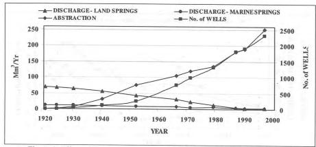
Figure 1: Effect of Groundwater Abstraction on Discharge from Springs [1, 5-9]
