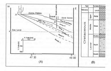
Figure 4(b): (a) Geologic cross-section and water flow, (b) Generalized stratigraphy.
