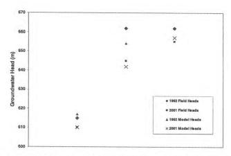
Figure 6: Comparison of field and model heads (m asl) at the three well group locations for 1992, and 2002.
