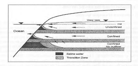
Figure 2: Salt/fresh water transition zone in multi-layered aquifer.
