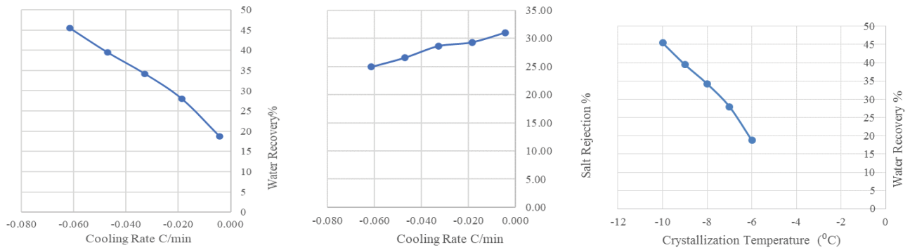
Fig. 7. Water recovery and salt rejection vs. cooling rate and water recovery vs. crystallization temperature at 70 min of crystallization time and flow rate of 10 L/min for 7 wt.%.
