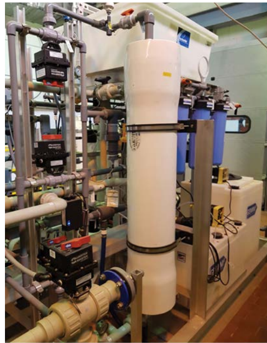
Fig. 5. Commercial scale FO module from Toyobo, Japan.
