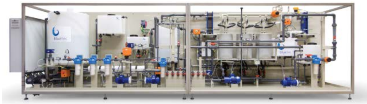
Fig. 7. Pilot scale FO-AGMD test unit.
