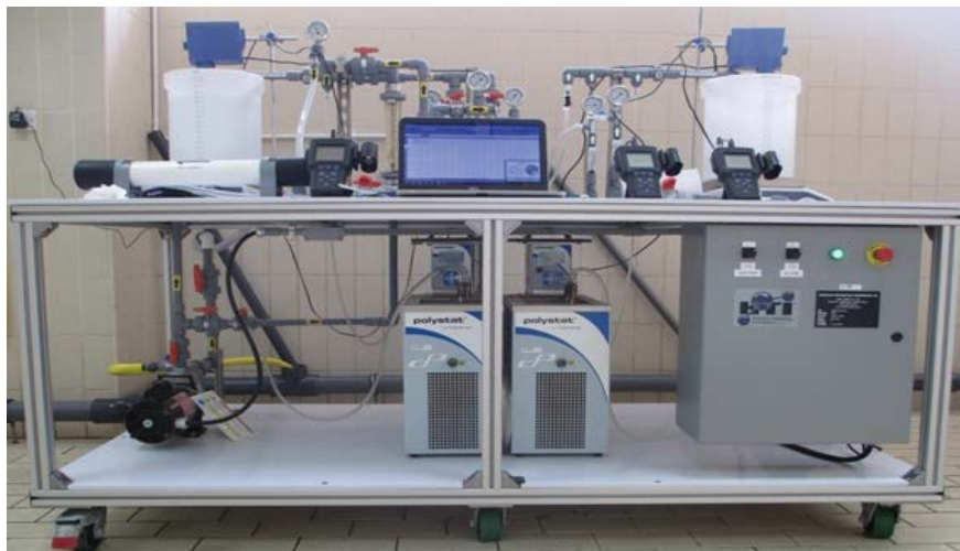
Fig. 3. Laboratory scale FO test unit.
